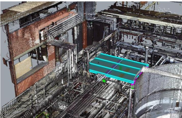
Point cloud of the space in BPL's plant where Courts Engineering custom-built a platform to take a 37-ton machine. The machine and the platform were lowered through the roof to fit precisely among the pipe network.
