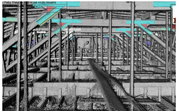
New roof trusses designed by Courts Engineering for Alexandra Palace. When inspecting the roof, Courts noticed targets on the walls indicating that scans had already been done; nobody else had been able to use the data.
