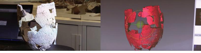
A Physical to digital: 3D scanning the basket pot using the HDI Advance (left photo). 3D representation on screen (right photo).
