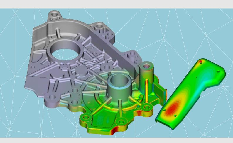
CAD based Scan Data Industrial 3D metrology software With innovative advances in 3D scanning technology, engineers are now able to leverage 3D pointcloud data that exceeds traditional measurement methods. (e.g. CMM,, etc.)
